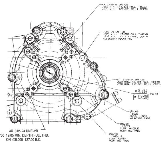
To make the center line of crankshaft the same as 190000 Model Series, order 695154 spacer kit.
